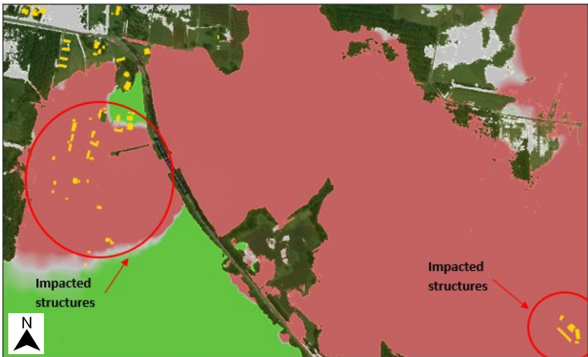
Figure 6: Floodplain impacts of Alternative 5 at Merricks Creek
