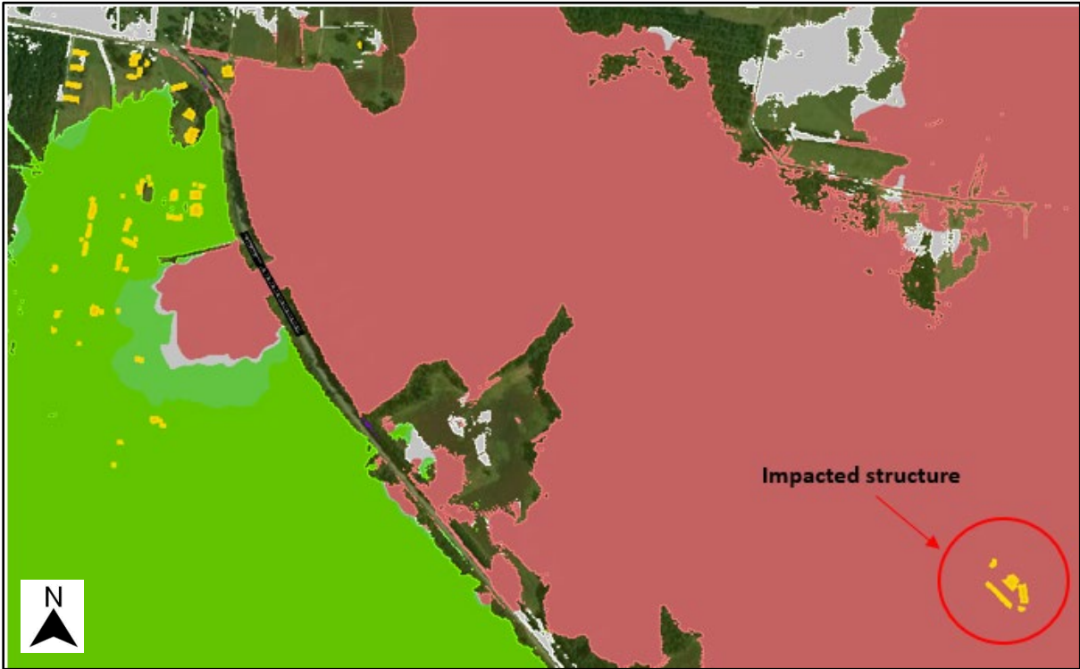
Figure 5: Floodplain impacts of Alternative 1 at Merricks Creek.
